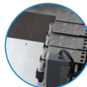
Cutting by multi cutting heads up to max.4pcs
